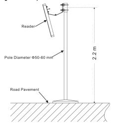
Figure 1: 1-shaped Stand Bracket Side-Loaded
